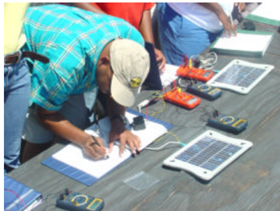
. . .then record the current and voltage. Repeat.
