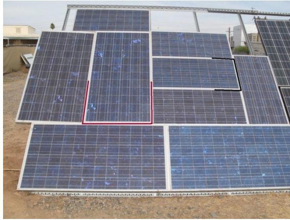
Figure 1: LMA (red border) and SMA (black border) mounted on an open rack for NOCT testing
